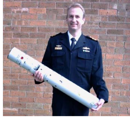
Figure 2 – Standard ‘A’ size sonobuoy, 3 ft in length by 5 inches in diameter, up to 18 kg (39 lbs) in weight
